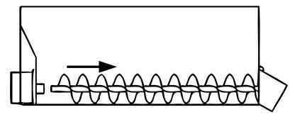
STEP 6: Pull up and slide the auger toward the motor end of the bucket until the auger is free of the discharge casing.
