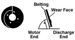
Install all rubber discs with the wear face toward the discharge end of the bucket.
